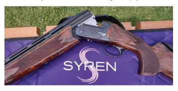
manufacturer and model. The barrel selector is designed in typical Italian fashion, situated atop the tang mounted safety. The action of this model is of traditional underlug design, the sample locked up very tight. The ejectors were strong and well timed.
