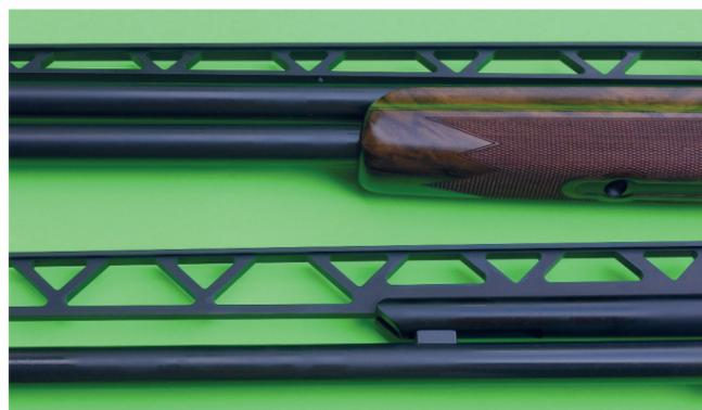
the Axis. Fabarm developed this technology some years ago – which they call TriBore. In front of the chamber the dimension goes immediately to .737 and stays at .737 for about half the barrel. Then starts a very slow taper to .730 to just shy of the screw choke threads. TriBore thus treats the shot pellets very gently – resulting in fewer pellet fliers that will quickly exit the effective pattern. This inner barrel
