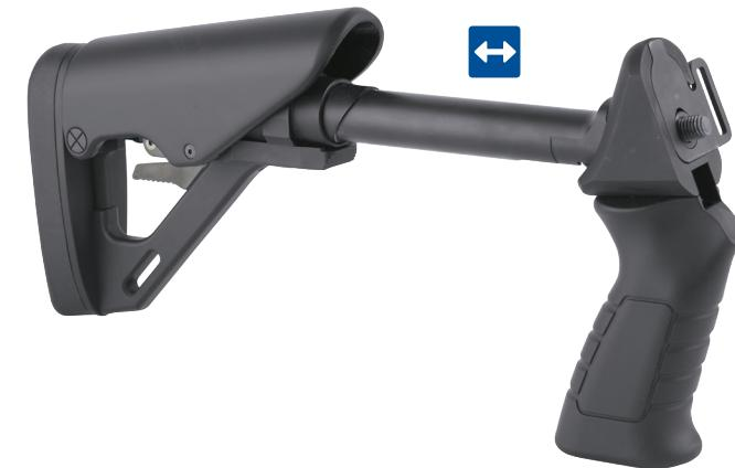
**EN** The STF/12 TELESCOPIC is using a collapsible stock with 6 optional length positions and an adjustable cheek rest. Its length-of-pull dimensions from mm. 250 to mm. 360 (9,84" to 14,17") give the opportunity to find the optimum adjustment for the use. Made from polymer composite and Aluminum 7075 it is precise, ambidextrous and integrates a sling swivel connector. Available in black or flat earth colours.
