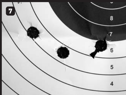
1_ 95 mm 3-shot group at 50 meters (54 yards) using the iron sights, a front rest and 28.5-gram Mirage Magnum ammo.
