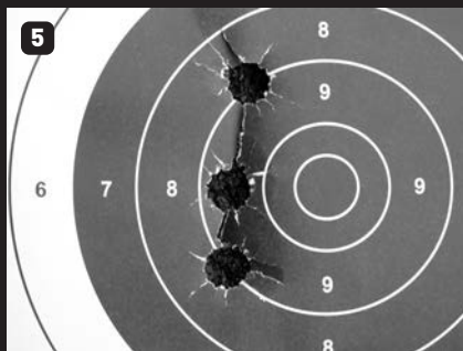
1_ 95 mm 3-shot group at 50 meters (54 yards) using the iron sights, a front rest and 28.5-gram Mirage Magnum ammo.
