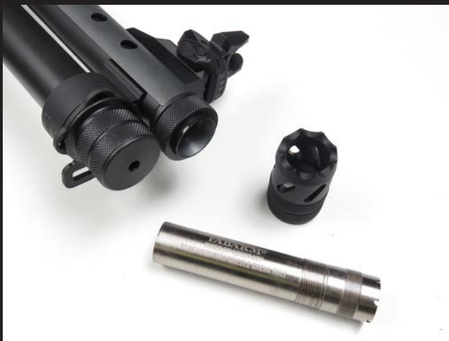
The barrel has a Tribore HP internal profile and is equipped with an Accuracy removable choke that can be used to mount the aluminum muzzle brake. The front sling swivel can be positioned at 3, 6, or 9 o'clock.
