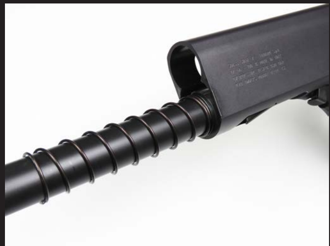
The magazine tube is made of aluminum instead of steel, to improve the balance of the gun. The spring that automatically pushes the fore-end forward can be easily removed if the user doesn't want to use it.
