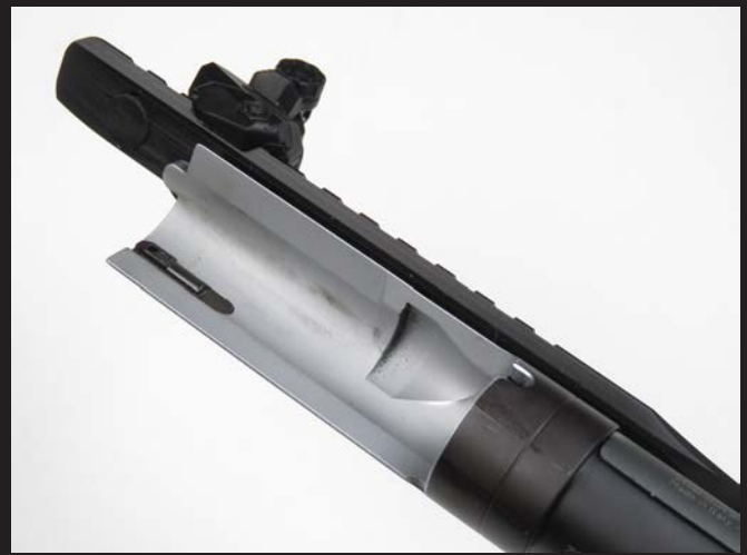
The breech extension, with the recess for the locking lug and the ejector. On the rear of the cantilever rail there is a rubber pad that prevents the receiver from getting scratched while mounting the barrel.
