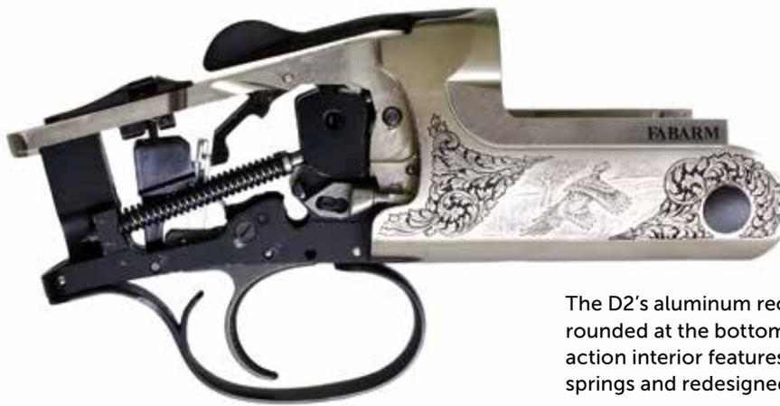
The D2's aluminum receiver is rounded at the bottom, and the action interior features improved sear springs and redesigned hammers.
